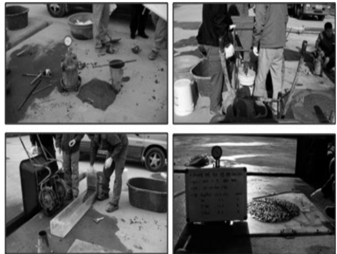
Figure 2. Consistency test of fresh concrete
