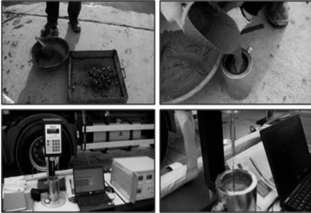
Figure 3. Rheology test for mortar separated from concrete
