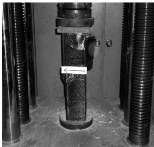
Figure 5. Horizontal reinforced specimen (CR3-A)
