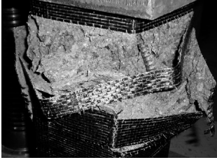
Figure 9. Horizontal reinforced specimen (CR3-A)
