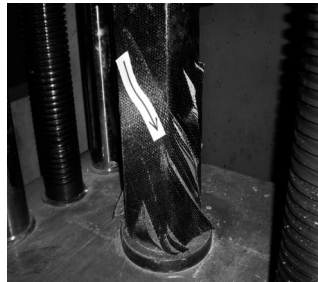
Figure 4. Inclined reinforced specimen (CR2-A)
