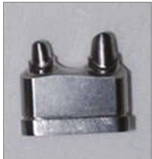
Fig. 2. Replica models with titanium block. This was fabricated with CAD/CAM system (Addtech Co., Seoul, Korea), and replicated master models.
