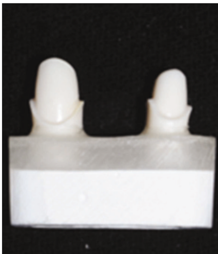
Fig. 1. Master model for replication with titanium block: Used dentiform teeth with 1.0 mm deep chamfer margin and 12 degree axial wall.
