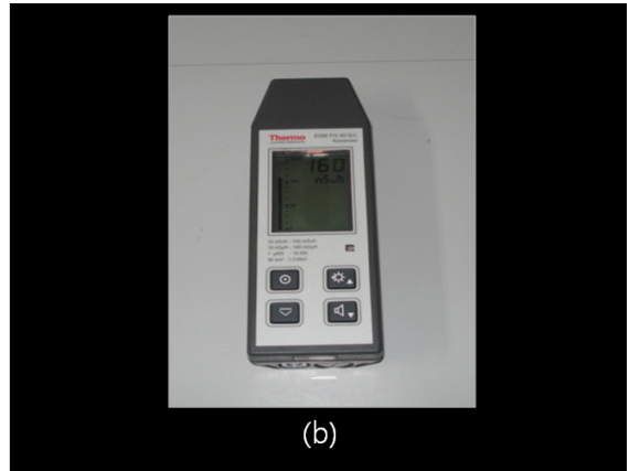
Fig. 2 This picture shows (a) Abdominal phantom lied on the 80cm height from the bottom and beside the center of the table (b) Radiation detector (FH 40GL)
