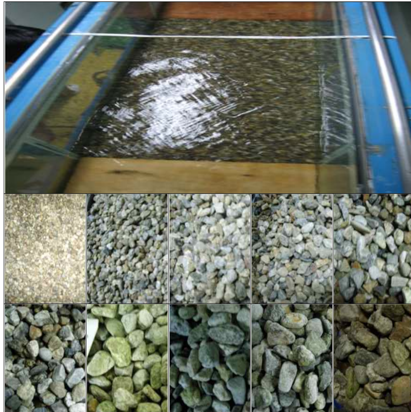
Fig. 2. Experimental Situation and Riprap Used for Experiment
