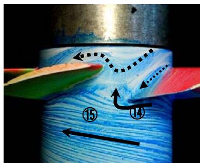
Fig. 10 Limiting streamlines of rear rotor operated without front rotor at Q=28 L/s
