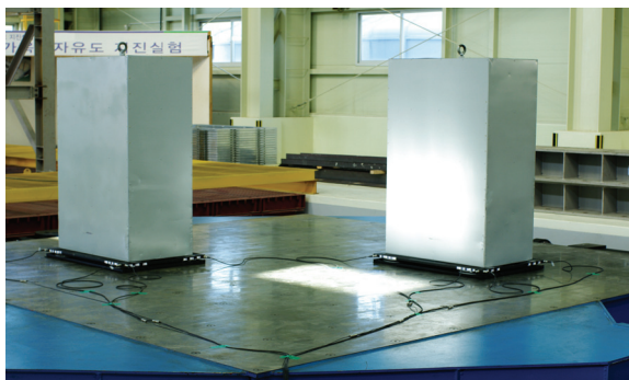
Fig. 14 CFPBS and accelerometers arrangement for shake table test
