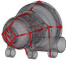
Fig. 10 Turbo blower modal geometry
