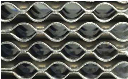
Fig. 1. Multi-stacked cross corrugated heat exchanger, hard to install temperature sensors to measure temperature of wall and fluid in the complex channel.
