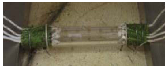
Fig. 8. Electrical interconnection of RTD temperature sensor array to the high temperature electrical wires.
