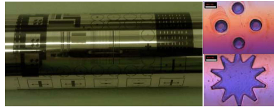
Fig. 3. Patterning of the developed dry film photoresist on the curved surface.
