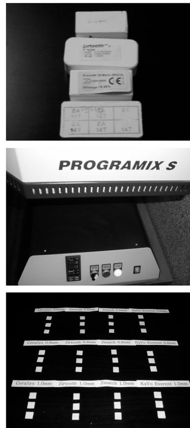
Fig. 1. Zirconia block & 0.4mm, 0.6mm, 0.8mm thickness Zirconia specimens
