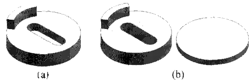
Fig. 6. Application of selective volume decomposition to a depression feature: (a) solid model with a slot. (b) two subvolumes generated by selective volume decomposition.
