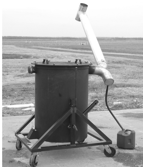
Fig. 1. Field scale biomass pyrolyzer developed by University of Missouri Delta Research Center. Pyrolysis converts crop biomasses in the reactor (i.e., 0.33 m 3 ) that is run at 400-500°C for 3-4 hours produce each batch of biochar. Note the air intake on the lower left of the reactor and the exhaust chimney above. The container on the right is catching the bio-oil.
