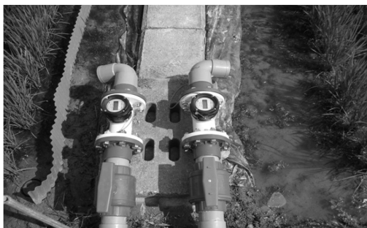
Fig. 1. Digital meter for measuring the amount of irrigation water.
