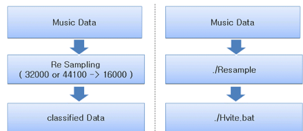
Fig. 3. GMM testing process for vocal and non-vocal classification.
