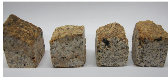
Figure 2. Decayed granite samples studied in this study.
