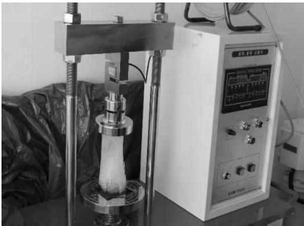
Fig. 5 Measurement of compressive strength for sea ice specimen
