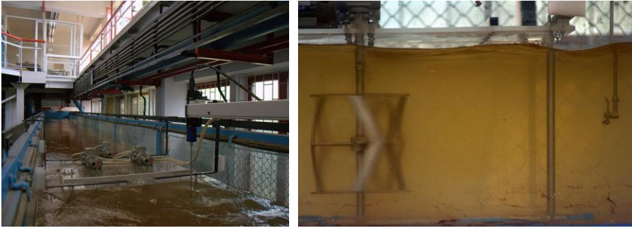
Fig. 7 Experimental set-up: Variable slope open channel, with turbines in an isosceles triangular arrangement pointing upstream, viewed from downstream (left); Acoustic Doppler Velocimeter sensor placed in the wake of the farm model (right)
