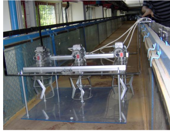
Fig. 2 Farm model at 1:5 scale, with 3 Achard turbines, here aligned on a row across the channel longitudinal axis (viewed from upstream)
