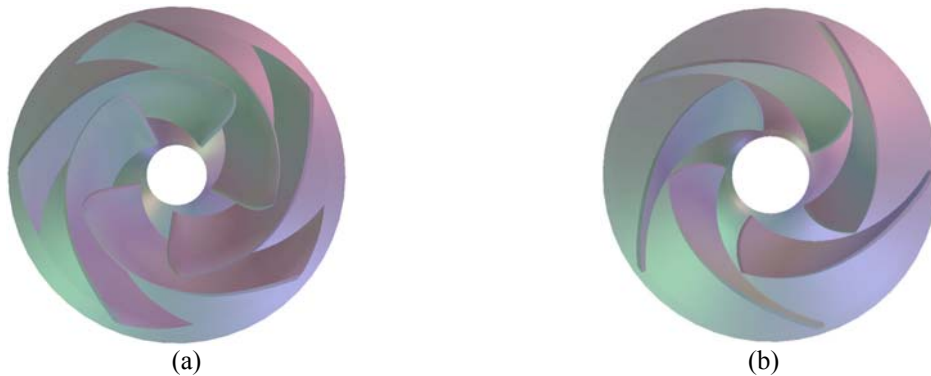
Fig. 16 Comparison of three-dimensional geometry; (a) Base design model of impeller; (b) Optimization model of impeller
