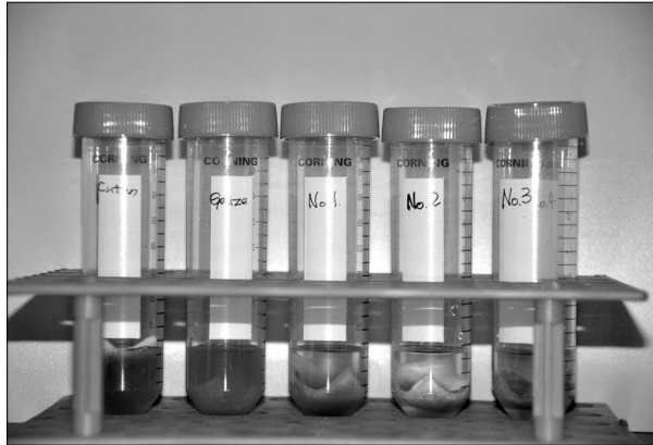
Fig. 4. In vitro blood compatibility test. 10mL of deionized water were carefully added by dripping water down the inside wall of the bottles without disturbing the clotted blood. The blood clotting test was carried out by spectrophotometric measurement.
