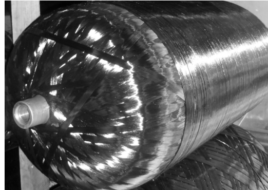
(b) Pressure container wrapped with a carbon fiber in hoop and helical directions
