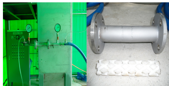
Fig. 2. View and structure of inline mixer
