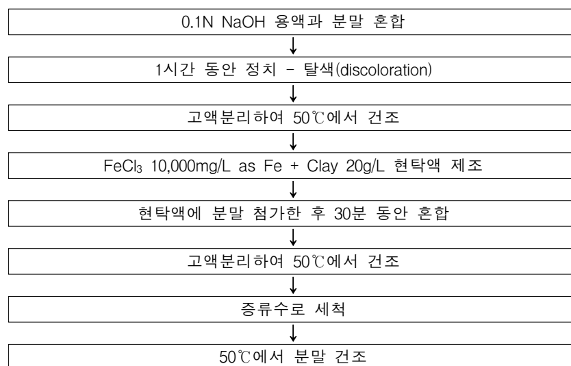
Fig. 2. Surface modification procedure for phosphorus removal.
