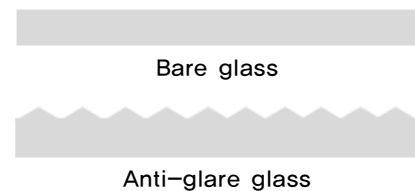
Figure 3. Cross section view of bare glass and anti-glare glass.
