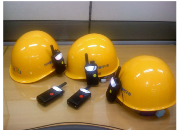
Fig. 6. Result of the prototype safety helmet for railways with bone conduction method.
