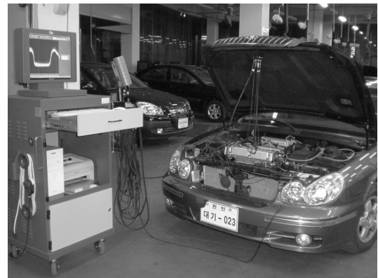
Fig. 1. Engine tune-up tester for pulse form on vehicle engine control
