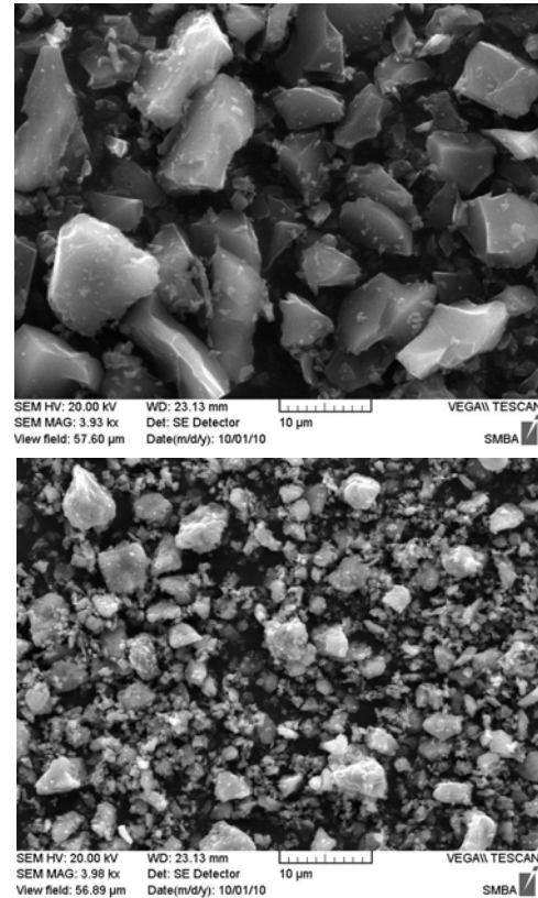
Fig. 1. FE-SEM image of ACF & \text{LiFePO}_4 .
