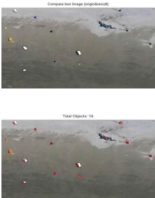
Fig. 8. Result of detection for marine debris using proposed method.
