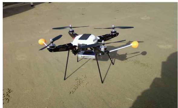
Fig. 2. The RC helicopter equipped with digital camera in gimbal mount for aerial photography.
