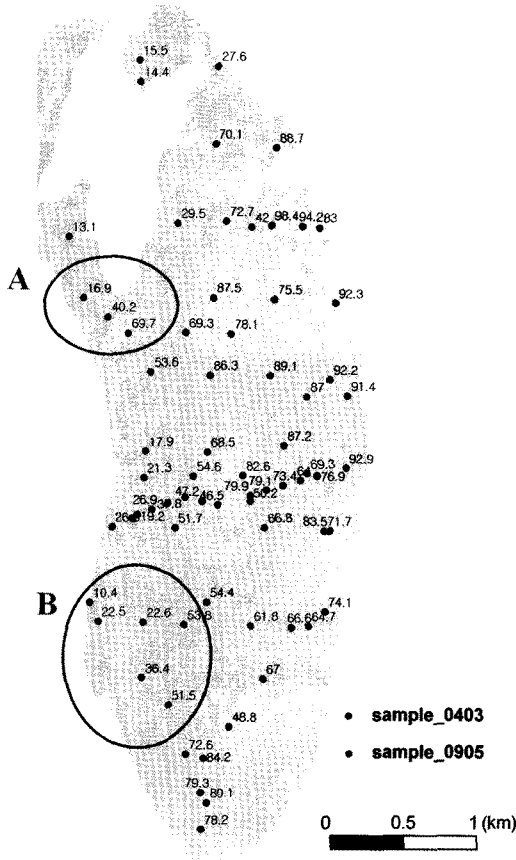
Fig. 4. Locations where the mud flat facies changed into the mixed flat facies (area in pink) overlaid with the sampling positions acquired on March, 2004 (points in red), and May, 2009 (points in blue) with the percentage of grains larger than very fine sand (0.0625 mm).
