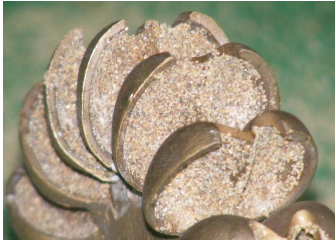
Fig. 6 Closer view of Pelton runner after pasting sand
