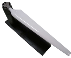
Fig. 1 Blade cantilever system
