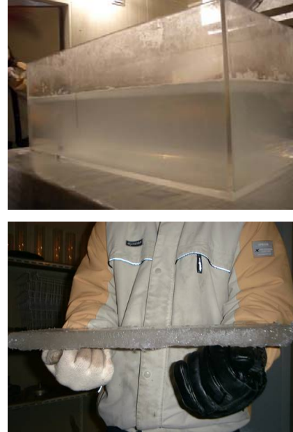
Photo. 1 Model ice sheet grown in the miniature ice tank
