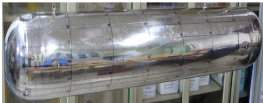
Fig.2 Points of the circular cylindrical shell marked on the surface
