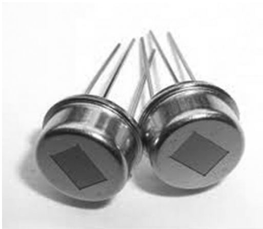
Fig. 1. Fabricated pyroelectric PIR infrared sensor.
