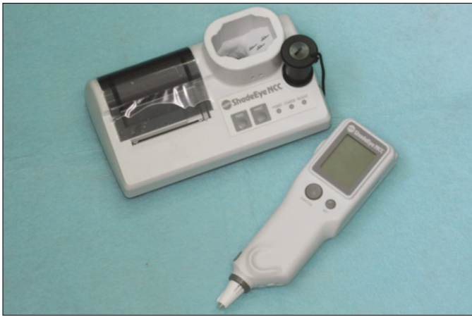
Fig. 2. ShadeEye-NCC® dental chroma meter (Shofu Dental, Kyoto, Japan).
