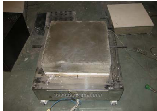
Figure 3. Simplified heating test set-up of specimen
