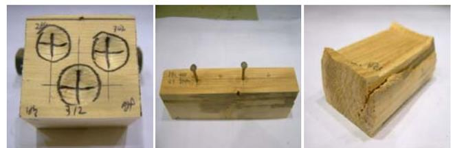
**Figure 12. After Durability Test of Flame Resistance Treated Compressed S.P.F.**
