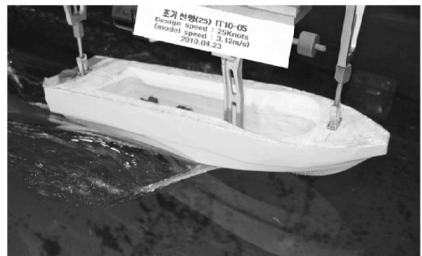
(a) Scaled initial hull(25) (Model number: IT10-05)
