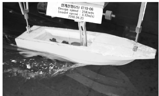
(b) Designed hull(25) (Model number: IT10-06)
