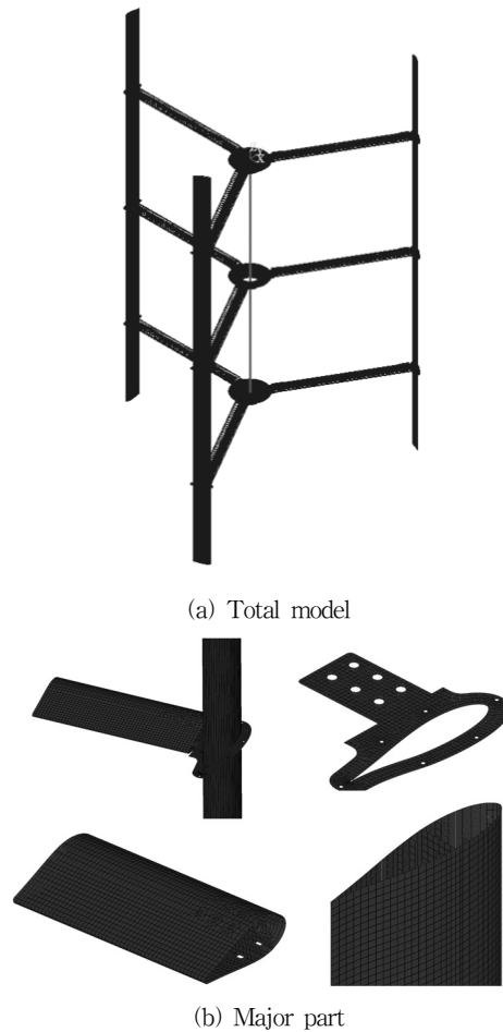
Fig. 9 Finite element structure analysis model
