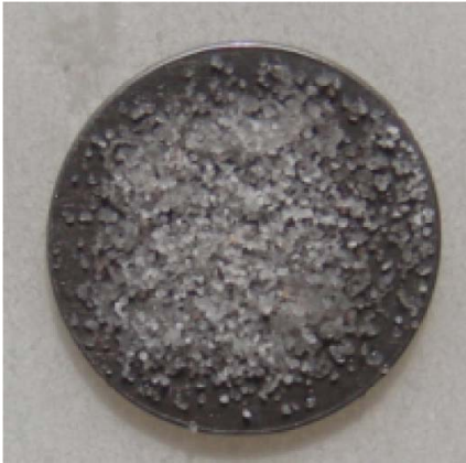
Fig. 1. Quartz sample loaded on stainless steel disk of 1 cm diameter. The sample consists of 2,000~3,000 quartz particles of 90~250 micrometer.
