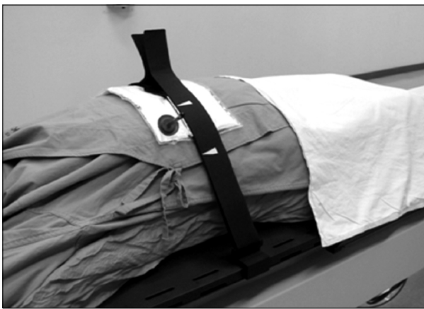
Fig. 1. The developed abdominal compression belt.
