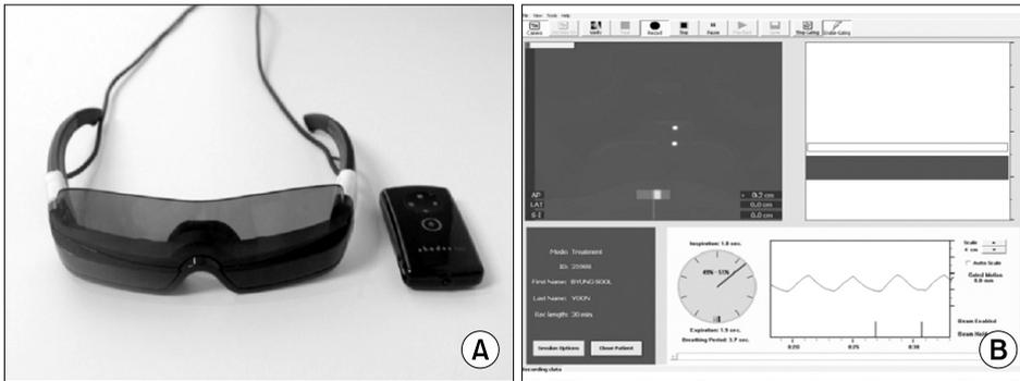
Fig. 3. Respiration acquisition system. Head-mounted display goggle (A), RPM respiratory gating system 1.7 software (B).
