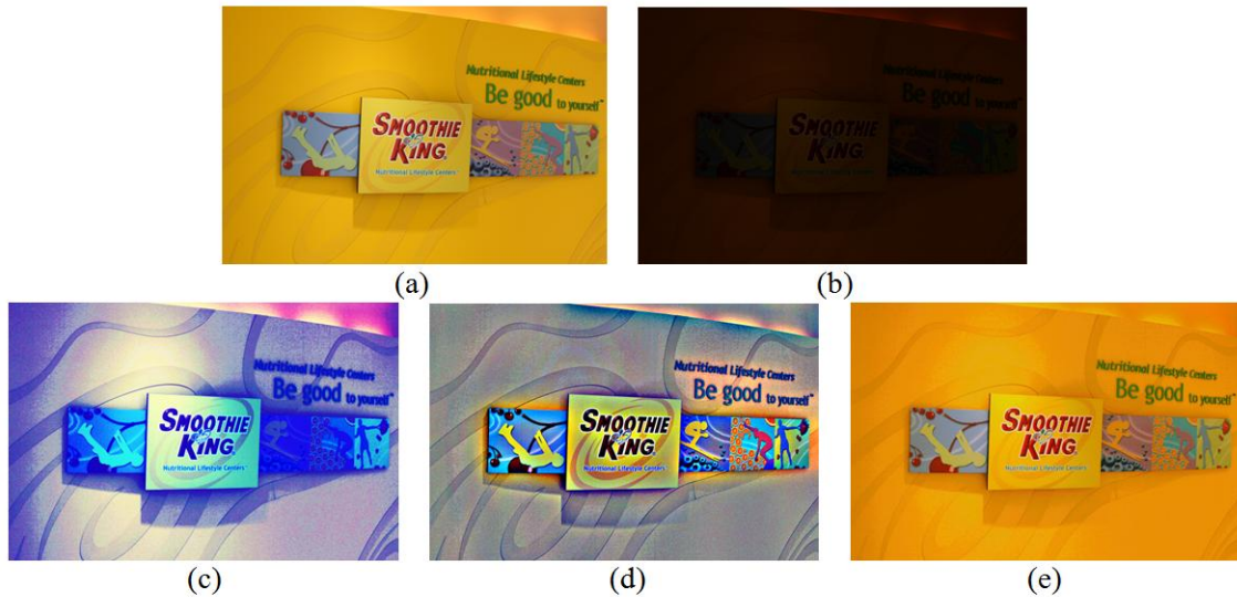
Fig. 9. Experimental comparison of the proposed method with the existing methods (a) image taken with proper EV indicated by an exposure meter in the digital camera (b) is an image taken with +4 EV from the proper EV. (c) is a result image of (b) by using color histogram equalization method. (d) is a result image of (b) by using multi-scale retinex with color restoration method. (e) is a result image of (b) by using the proposed method.
