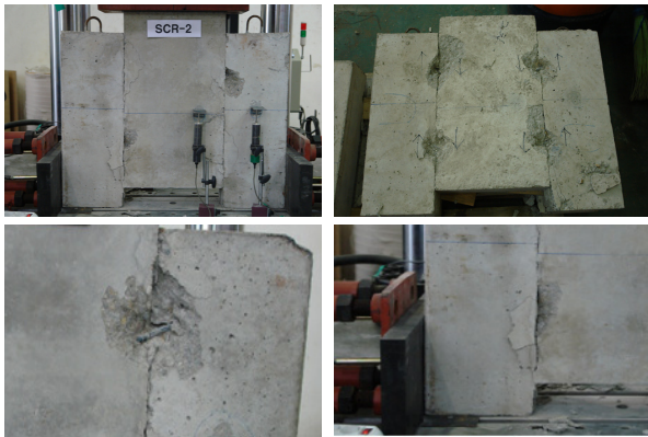
(a) Failure shape of specimen (SCR series)
