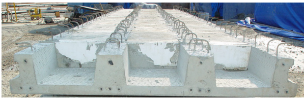
Fig. 2 Section shape of Rib-plus PC slab
