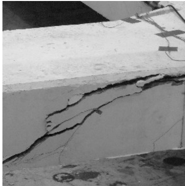
Photo 4 Crack pattern of specimen 1 at failure
