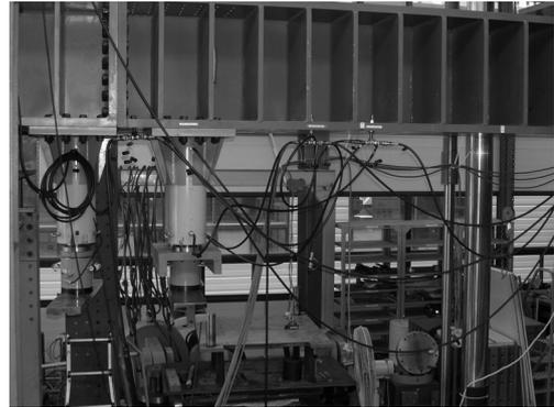
Fig. 7 Installation Sight of Oil Jacks
