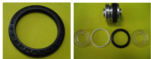
(a) Piston seal (b) Piston seal assembly Fig. 2 Photo of piston seal and assembly
