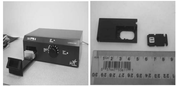
Figure 3. Landauer InLight™ microstar reader and OSL detector
