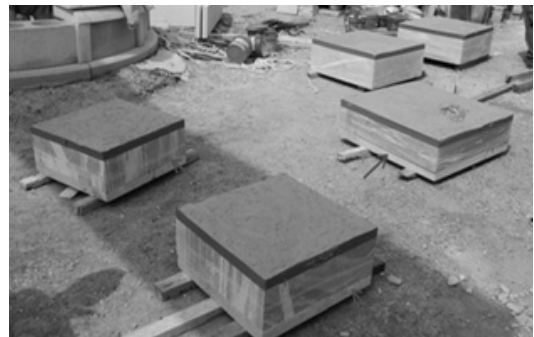
Fig. 3. A photograph of anisotropic rock specimens for LCM tests.
