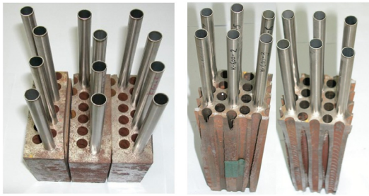
Fig. 4 Tube specimens prepared by expanding (a) explosively, and (b) hydraulically
