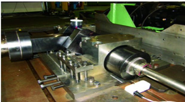
Fig. 14 An example of crankshaft type torsion fatigue bar test system
